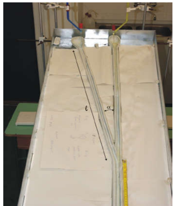
Figure 4. The hydrophilized rinnenkarren system built up to measure the flow of water. [4] Legend: \alpha . joining angle of the secondary channel, l . the length of the secondary channel
