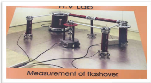
Fig. 3. Flashover voltage test arrangement
