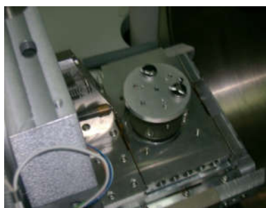
Figure 3. The two sampleholders placed in the analysis chamber
