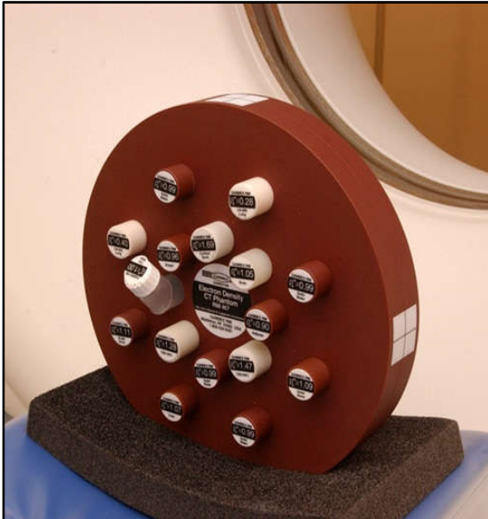
Figure 1. GMMa phantom with multiple density plugs on treatment modality bore
