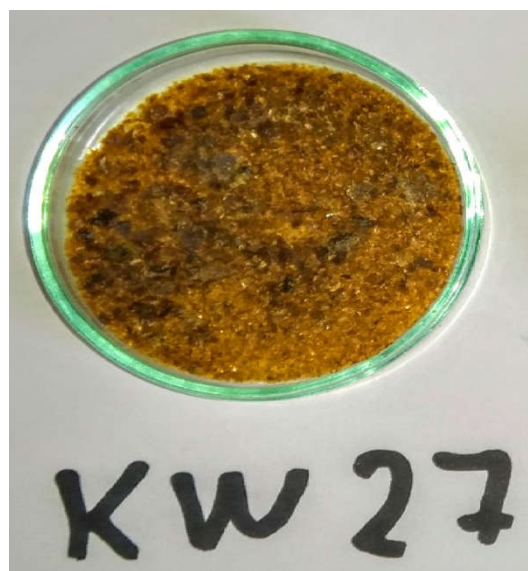
Fig. 1. Patri dish containing the dead biomass of Nocardia sp. Kw 27. that is used to biosorption of Cu 2+ , Pb 2+ , and Cd 2+ from aqueous solutions
