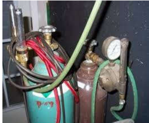
Plate 2. Shielding gas cylinder and regulator
