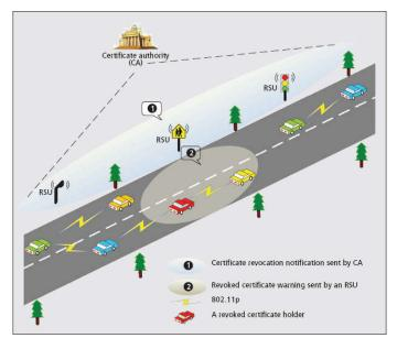
Figure 2. Area consisting of RSUs and moving Vehicles
