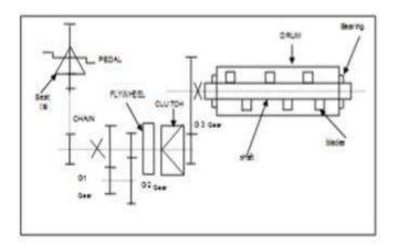
Figure 1. Schematic arrangement of a Nursery Fertilizer mixer machine
