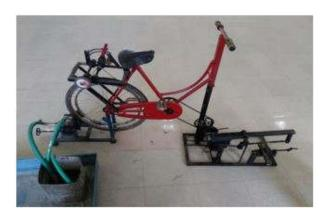
The machine comprise of various linkages, sprocket, chain drive mechanism and pedal assembly on which force is applied by an operator which indirectly convert the pedaling power into working stroke of hacksaw, which is 60 stroke/min and can cut 30mm diameter work piece of various materials like wood, PVC, plywood, hollow metal pipes and bars. Also the water pump can lift up the water from 10m to 16m by attaining speed up to 1890 to 1900 RPM. The DC motor can generate 12 v of
