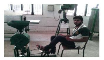
Figure 3. Pedal Operated Flour Machine
