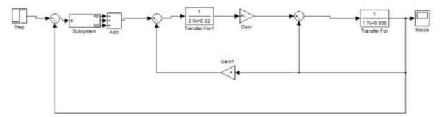
Figure 4.The diagram of Fuzzy-PID and PSO-PID Controller dc motor
