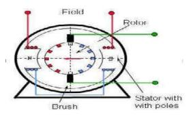
Fig. 1. Basic diagram of DC motor
