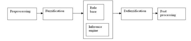
Figure 2. Arrangement of fuzzy logic controller
