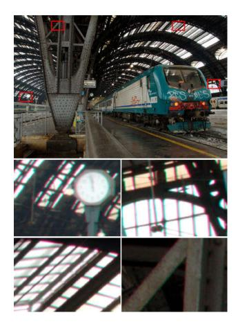
Figure 8. Cropped sections exhibiting LCA
