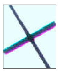
Figure 7. Lateral chromatic aberration (LCA)
