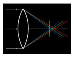
Figure 2. Axial or longitudinal chromatic aberration (ACA). Focal length varies with color wavelength
