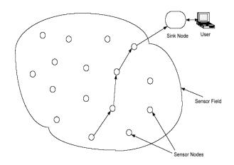
Fig 1.1. The basic structure of Wireless Sensor Networks
