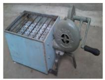
Fig. 1. The Improved Barbecue Stove: It was designed with features to minimize the stress on arms, probability of accidents and improving the performance of the stove. The stove is in cubical shape with insulations to avoid the direct contact of heat to the body and the provisions were made to avoid the contact of fire with the body part (fingers). Instead of making use of hand fan, a blower was attached to the model to reduce the stress produced by constant fanning
