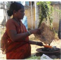
Fig. 2. Vendors performing the experiments: To test the performance of the barbecue stove, the experiments were carried out taking charcoal as source of fuel. The time and fuel consumption in barbecue stove was calculated during the process of roasting and the results were compared with that in conventional stove. Five corns were taken as a standard since the barbecue stove had the provision of cooking five corns at a time
