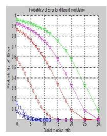
Figure 1. Shows that probability of Error versus signal to noise ratio for Different Modulation Technique
