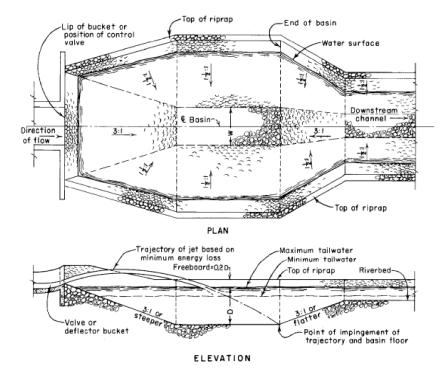
Fig. 1. Plunge pool energy dissipater (Design of small dams 1987)
