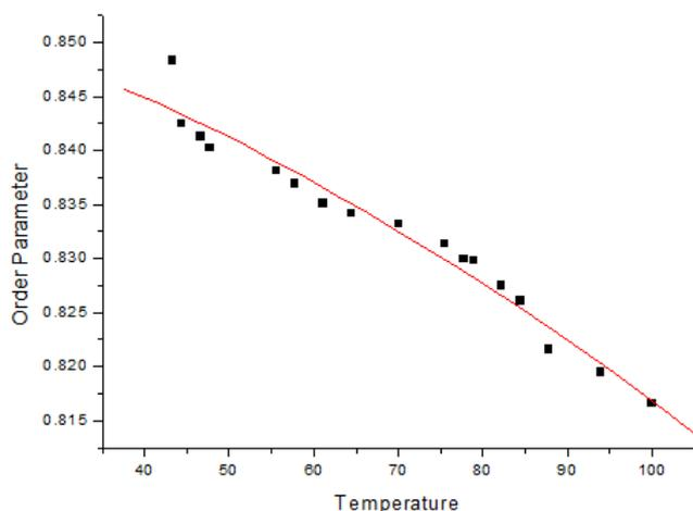
Fig. 4. Variation of order parameter with temperature for 1d<sub>3</sub>CC
