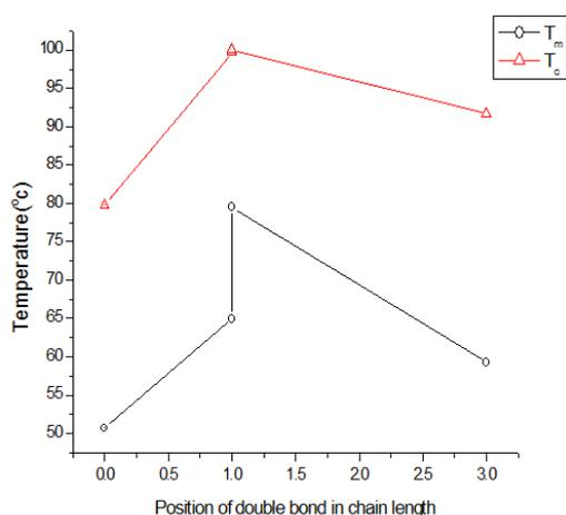
Fig. 1. Variation of thermal stability with the position of double bond in alkenyl chain length
