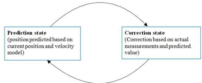
Figure 1. The basic concept of the Kalman tracker
